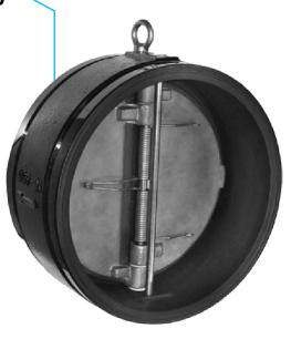
The Fig. CV890 Dual Disc Check Valve is a grooved end, dual disc check valve used for pipelines to convey water and other fluids with a rated working pressure up to 300 psi (20.7 bar). This Dual Disc Check Valve is available in sizes from 14 inches (350 mm) to 24 inches (600 mm).
